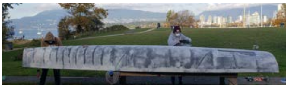
Smoothing out Raye ’s carbon fibre hull with sandpaper to get it ready for painting
