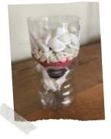
**STEP 9**  $\rightarrow$  Test your water filter by slowly pouring the water onto the pebbles at the top of your filter. Watch the water as it passes through the layers and exits your filter looking much cleaner! Remember that your water is not safe enough to drink, even if it looks clean!
